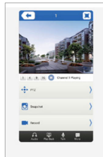
4. Real-time monitoring: Support PTZ, Snapshot, Record, Audio, Play Back etc. function
