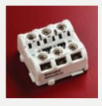
The Mini Monitor Module is an interface within an entirely new housing. This allows the unit to be fitted onto a standard 35mm DIN-Rail (using a twist-click motion) or mounted within an enclosure, such as a Pull Station. It is designed to monitor the state of one or more single pole, voltage free contacts connected on a single pair of cables and to report the status to Apollo compatible analog control equipment.
